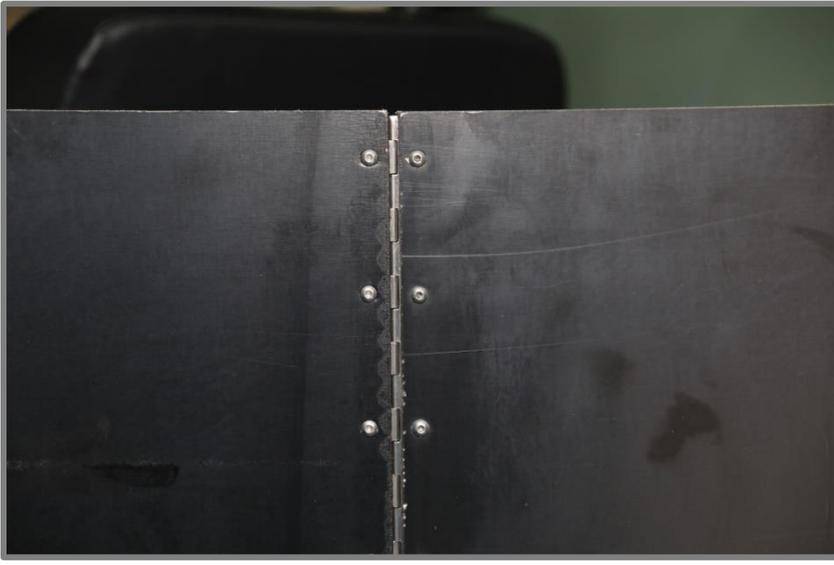
6. **Be very careful when handling the Roof Locker hinged sections as I have left a gap under the hinge to allow for the hatches to not only fold down, but also to fold partly upwards towards the roof when closing and inserting the locking tube under. It would be very easy to trap your fingers in the gap underneath when handling – you have been warned!**
