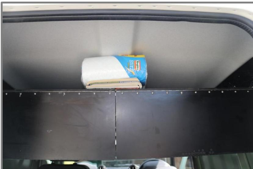
7. With the locking bar removed, slide the two sections into place, one at a time with the close fitting gap to the middle and the larger gap on the outside which allows some space to miss the locking plates and setscrew heads. Position these two sections so there is an even parallel gap each side between them and the roof sides. **The underside back of**
