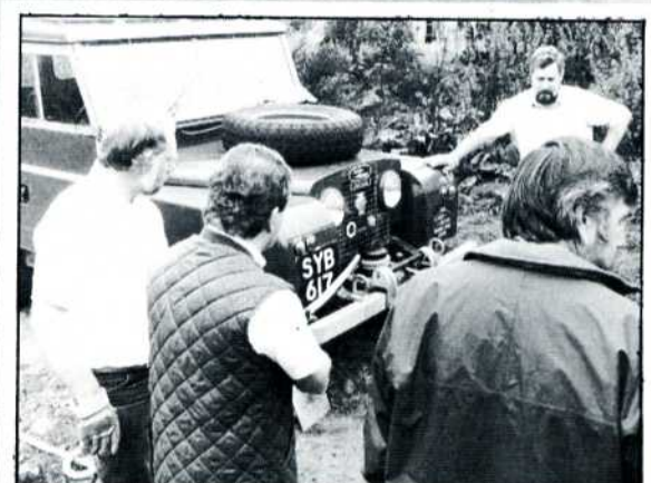
David Bowyer watches in the background while LRO's John Cornwall operates the capstan winch on David's Series I.
