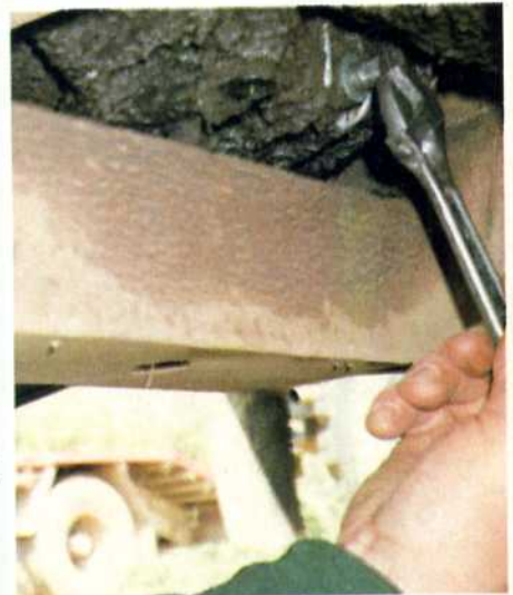
The 'wading' plug has to be fitted into the clutch housing and must be removed afterwards for normal road use.
