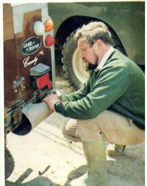
Mud flaps need to be tied up to keep them from harm, wing mirrors put in, aerials down, batteries secured and tyre pressure down to about 20psi. Before setting off free-wheel hubs must be engaged and four-wheel-drive low ratio, selected.
