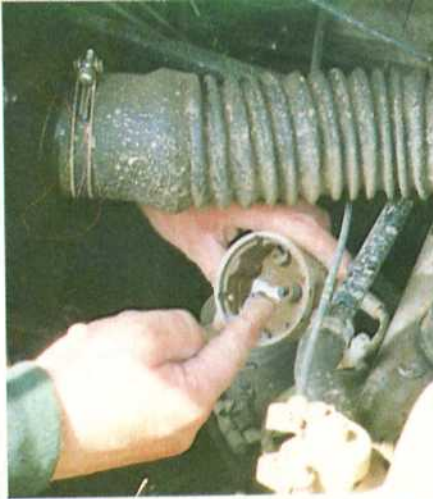
Next came preparation of the vehicles, which starts with silicone grease around the distributor cap seal.
